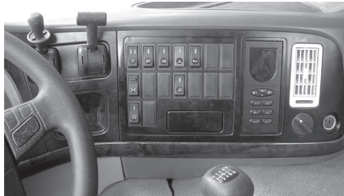
1.Hand brake handle 2. Trailer hand brake handle 3.Rocker switches 4. Air conditioner control panel and display 5.Horn switch 6. Steering wheel 7. Gearshift lever handle 8. Cigarette lighter
