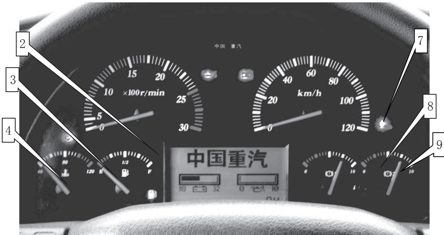
1 Tachometer 2.Information screen 3.Fuel gauge 4. Water temperature gauge 5.Speedometer 6.Air pressure gauge 1 7.Signal indicator 8.Knob 9. Air pressure gauge 2
