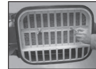
6. Assemble the filter core assembly. Install the upper filter core first and then the lower filter core, and finally tighten with rubber pad, flat pad and wing nut.
