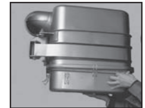
7. Assemble the lower housing. Fasten the lower housing to which oil is added with hook firmly.
